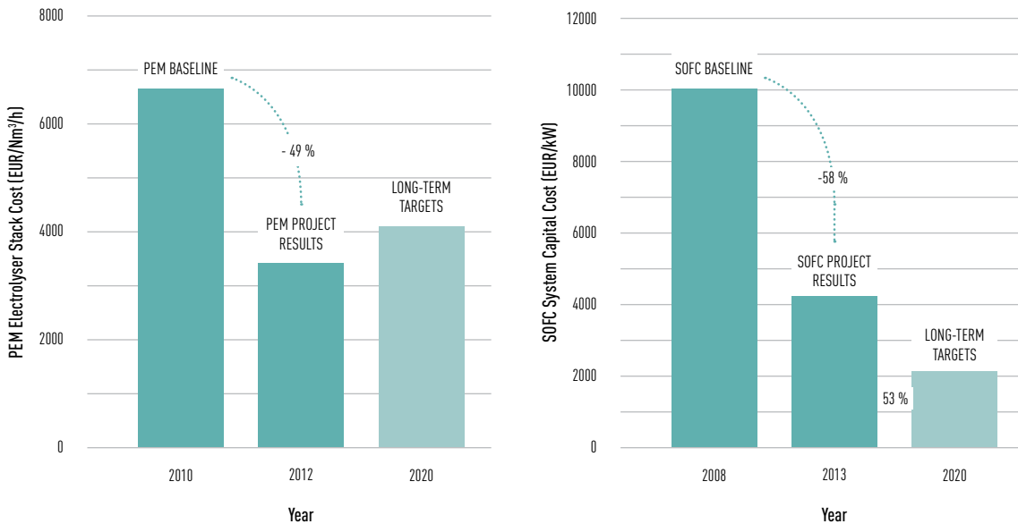
FIGURE 1.2.2 (C) | COST ACHIEVEMENTS FOR ELECTROLYSERS (LEFT) AND FUEL CELLS (RIGHT) UNDER FCH JU (2008–13)
