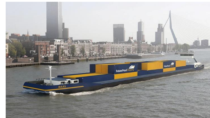
FPS Maas, retrofitted inland container vessel with 2x 500kg compressed hydrogen in swappable containers 1
