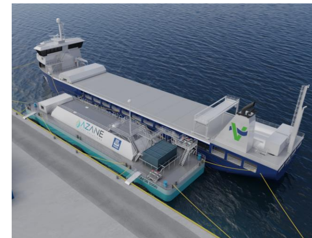
Ammonia bunkering infrastructure prototype by AZANE Fuel Solutions (Source: link )
