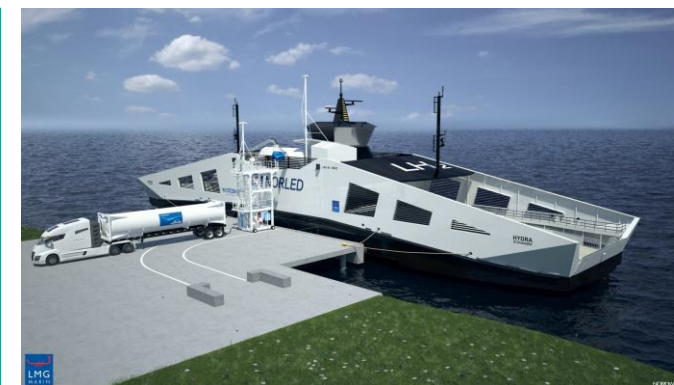
LH2 bunkering for MF Hydra through truck-to-ship 5
